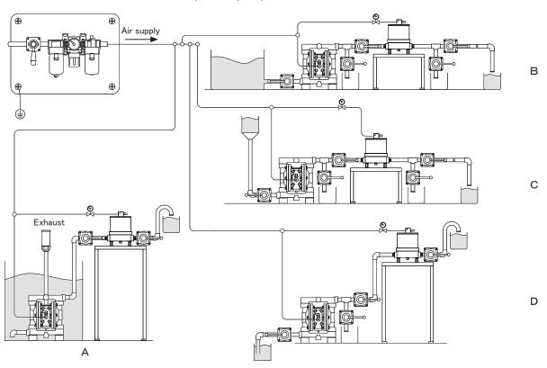
Please fix the dampener with anchor bolts in mounting holes.
