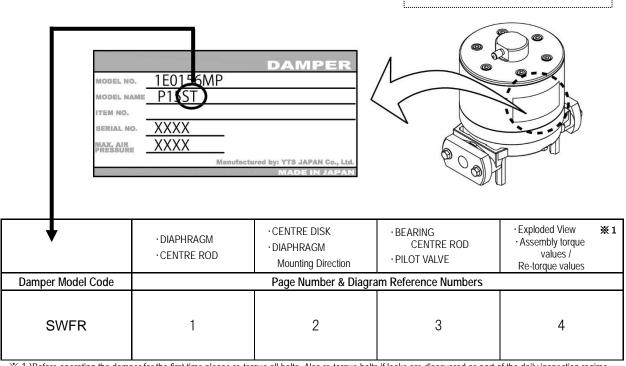
% 1 )Before operating the damper for the first time please re-torque all bolts. Also re-torque bolts if leaks are discovered as part of the daily inspection regime.
