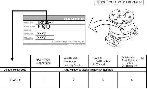
\* 1 )Before operating the damper for the first time please re-torque all bolts. Also re-torque bolts if leaks are discovered as part of the daily inspection regime.
