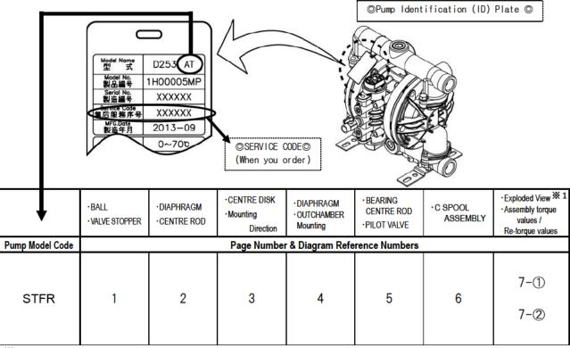
X1) Before operating the pump for the first time please re-torque all bolts. Also re-torque bolts if leaks are discovered as part of the daily inspection regime.
