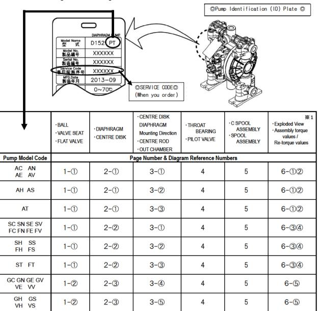
× 1 )Before operating the pump for the first time please re-torque all bolts. Also re-torque bolts if leaks are discovered as part of the daily inspection regime.
